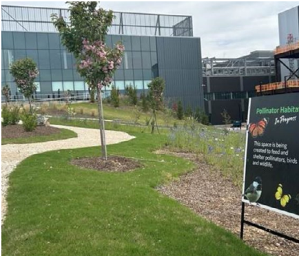
View of the rain garden, where native plants filter stormwater runoff before entering the drains
